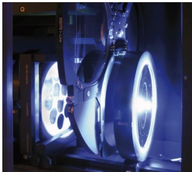
**FIGURE 6: MO Exposure Optics, a new illumination system for mask aligners based on microlens array homogenizers.**
