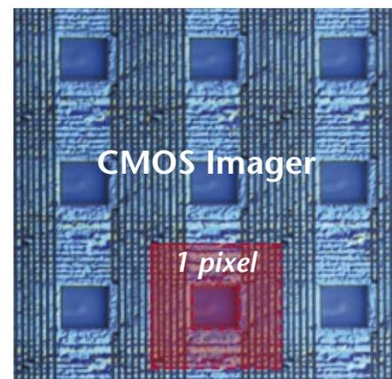
FIGURE 3: Microlens on CMOS image sensor to enhance fill-factor.
