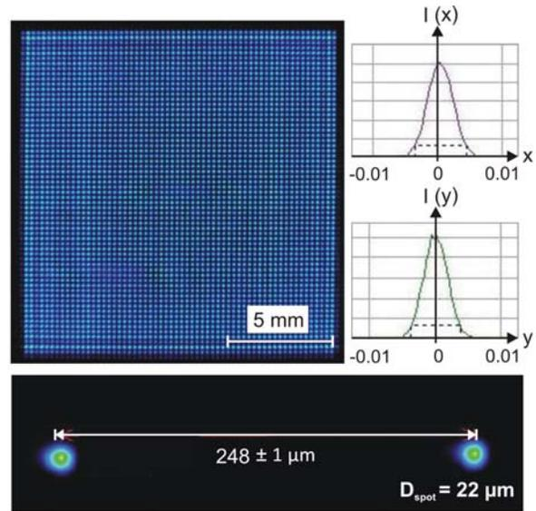
Fig. 4 Spot-Array generated with fly's eye setup
