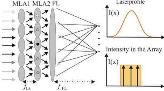
Fig. 2 Fly's eye condenser for flat-top generation
