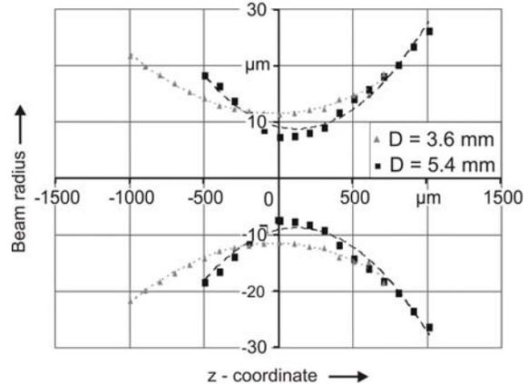
Fig. 5 Measured beam caustics for different collimated beam-diameters
