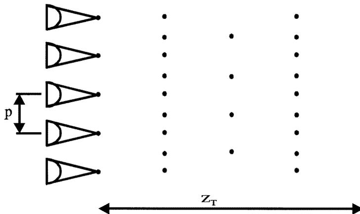
**Figure 1.** Illustration of the Talbot effect for the foci of an array of microlenses. In the  $\frac{1}{4}$  and  $\frac{3}{4}$  Talbot planes the number of foci is, for example, doubled whereas in the  $\frac{1}{2}$  Talbot plane the number of foci is not increased but the foci are laterally shifted by half a period  $p$ .  $z_T = 2p^2/\lambda$  is the Talbot length.
