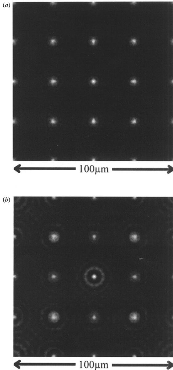
**Figure 2.** Simulation of the foci of a refractive microlens array in the  $\frac{1}{8}$  Talbot plane. Shown is one period of the array with  $4 \times 4$  multiplied foci. In (a) there are stops between the lenses whereas in (b) there are no stops between the lenses.
