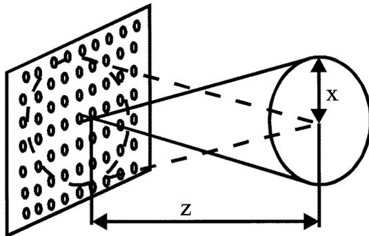
**Figure 4.** Illustration of walk-off effects. The intensity of light of one lens with numerical aperture NA at a distance  $z$  is decreased but the number of lenses which supply light to the foci in the fractional Talbot planes is increased.
