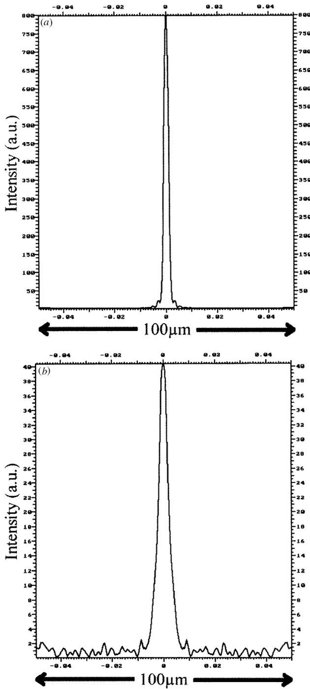
Figure 3. Simulation of the blurring of the foci in the 1 Talbot plane. (a) 0 Talbot plane (focal plane), (b) 1 Talbot plane.
