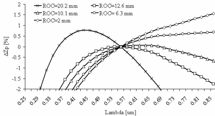
Fig. 9. Relative variations on  $Z_p$  calibrated at 550 nm for five microlenses of  $\varnothing = 635 \mu\text{m}$  for five ROC, illuminated by a plane wave at different wavelengths.
