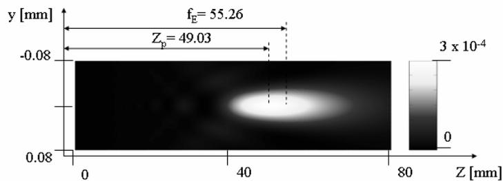
Fig. 3. Intensity (a.u.) distribution behind a microlens of  $\varnothing = 635 \mu\text{m}$  and  $ROC = 25.2$  mm illuminated by a plane wave at 633 nm. The lens stands in the  $x,y$  plan while  $z$  corresponds to the propagating axis.
