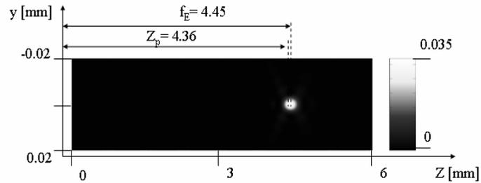
Fig. 2. Intensity (a.u.) distribution behind a microlens of  $\varnothing = 635 \mu\text{m}$ ,  $ROC = 2.03$  mm, illuminated by a plane wave at 633 nm. The lens stands in the  $x,y$  plan while  $z$  corresponds to the propagating axis.
