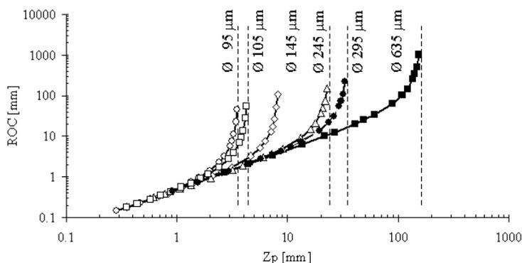
Fig. 6. ROC [mm] versus position of peak irradiance for six diameters of microlenses illuminated by a plane wave at 633nm.
