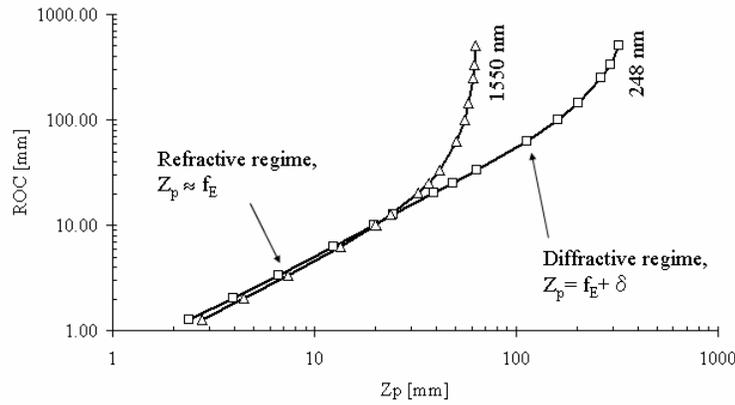
Fig. 7. ROC versus position of peak irradiance  $Z_p$  for microlenses of  $\varnothing = 635 \mu\text{m}$  illuminated by a plane wave at two different wavelengths.
