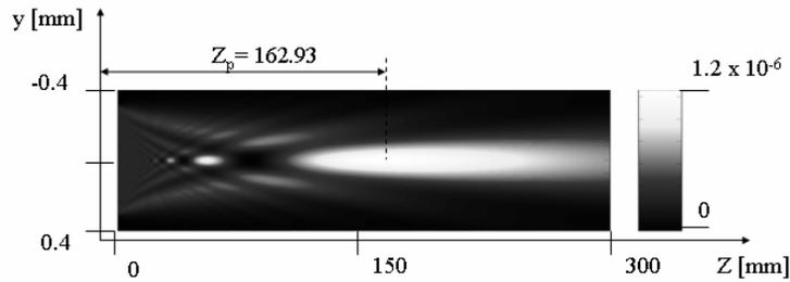
Fig. 5. Intensity (a.u.) distribution behind an aperture of  $\varnothing = 635 \mu\text{m}$  illuminated by a plane wave at  $633 \text{ nm}$ . The lens stands in the  $x,y$  plan while  $z$  corresponds to the propagating axis.
