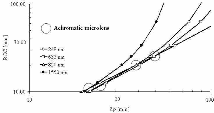
Fig. 8. ROC versus position of peak irradiance  $Z_p$  for a microlens of  $\varnothing = 635 \mu\text{m}$ , illuminated by a plane wave at four different wavelengths. The crossings between two curves corresponding to achromatic microlenses are shown with circles.
