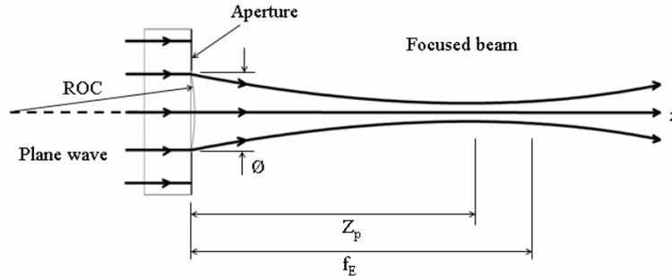
Fig. 1. Model of a plano-convex microlens illuminated by a plane wave.
