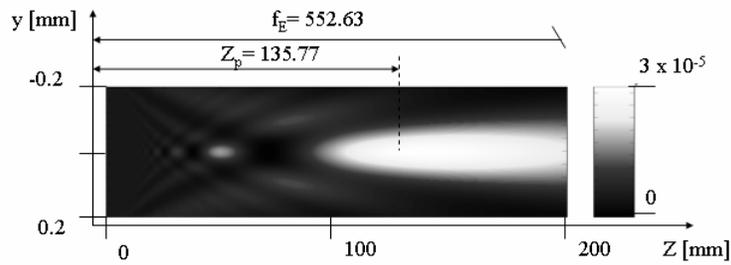
Fig. 4. Intensity (a.u.) distribution behind a microlens of  $\varnothing = 635 \mu\text{m}$ ,  $\text{ROC} = 252 \text{ mm}$ , illuminated by a plane wave at  $633 \text{ nm}$ . The lens stands in the  $x,y$  plan while  $z$  corresponds to the propagating axis.
