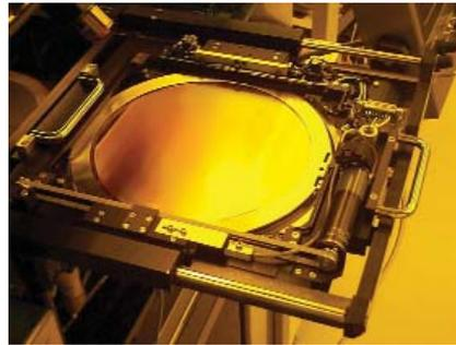
Figure 4: Ultra-flat microlens projection system integrated into the SUSS MicroTec MA150-MPL Mask Aligner. Microlens Projection Lithography allows photolithography on curved or non-planar substrates, in V-grooves, and holes.
