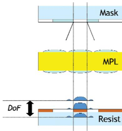
Figure 3: A microlens based projection system projects a photomask onto a resist layer. Each lens channel images a small part of the photomask pattern onto the wafer. The partial images overlap consistently and form a complete aerial image of the photomask. Front- and backside telecentricity provides equal line width over the whole depth of focus DoF.
