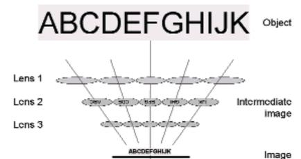
Figure 1: Miniaturized imaging systems based on spatial superposition of the partial erect images created by adjacent imaging channels. Each lens channel images only a limited angular section.
