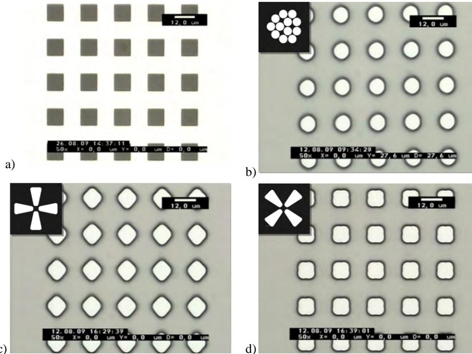
Figure 6. Experimental results for Mask Aligner Lithography using MO Exposure Optics and illumination filtering. Photographs of (a) photomask consisting of  $10 \times 10 \mu\text{m}$  large holes and (b) to (d) the resulting prints in  $1.2 \mu\text{m}$  thick photoresist exposed at a proximity gap of  $100 \mu\text{m}$  behind the photomask (a) using different illumination filter configurations shown in the small windows in the upper left corner of the photographs.
