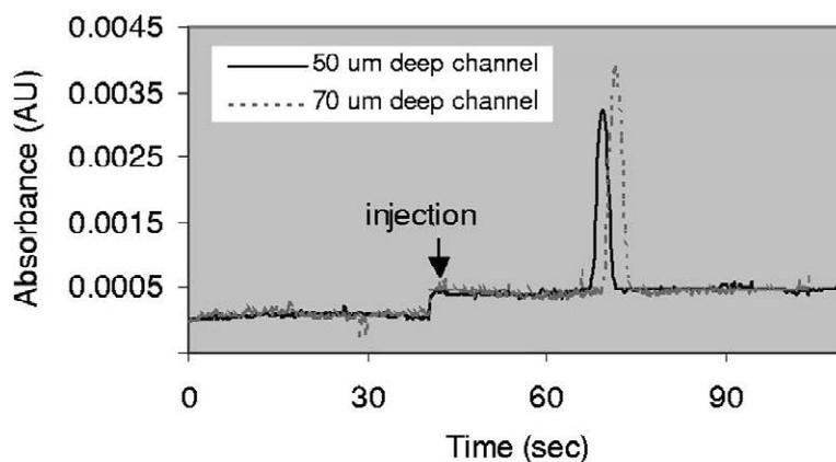
Fig. 3. UV absorbance peak of 0.1 mg/ml tryptophan through 50- and 70- $\mu\text{m}$  deep channels in different PDMS/quartz chips. Running buffer: 20 mM Tris-HCl, pH 7.6;  $E_{\text{sep}}$ : 400 V/cm;  $L_{\text{eff}}$ : 2.5 cm. The different migration times of the peaks are due to manual switching between injection and separation modes.
