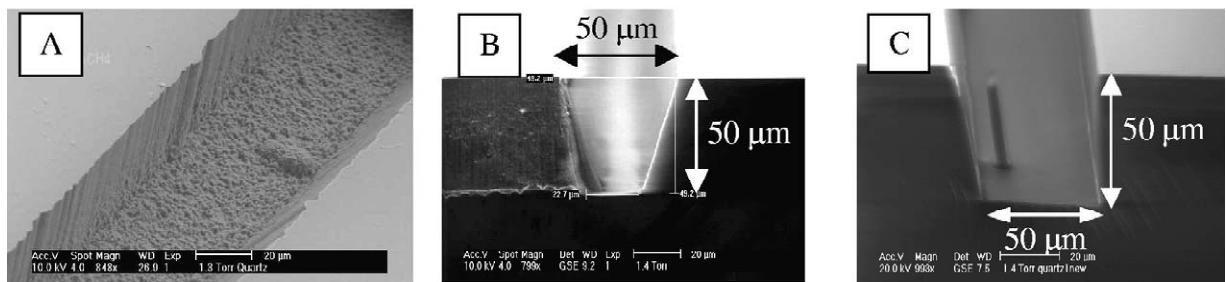
Fig. 2. ESEM photos of quartz channels (XL 30, ESEM-FEG, Philips). ICP–RIE process conditions: (A) Coil: 750 W, plate electrode: 50 W chamber pressure: 5 mTorr, 20 °C,  $\text{C}_3\text{F}_8$  gas with  $\text{CH}_4$ . (B) Coil: 750 W, plate electrode: 120 W, chamber pressure: 2.5 mTorr, 20 °C,  $\text{C}_3\text{F}_8$  gas only. (C) Coil: 750 W, plate electrode: 180 W, chamber pressure: 3.5 mTorr, 20 °C,  $\text{C}_3\text{F}_8$  gas only.
