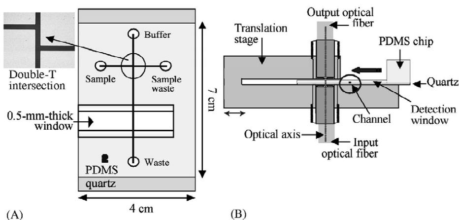
Fig. 1. (A) Top view of the PDMS chip containing channels for CE separations and a thin PDMS window for absorbance detection. The double-T intersection is presented in the insert on the left. (B) Cross-sectional view of the chip alignment with respect to the optical axis. The thin detection window is inserted between the two pre-aligned optical fibers.
