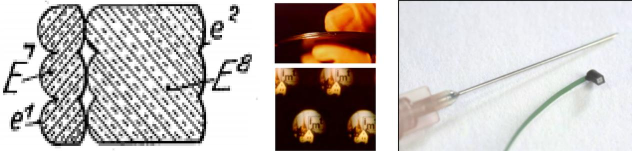
Figure 12. (left) Stack of double-sided microlens arrays as patented by Arnold Arnulf in 1932, (center) a stack of four 100mm microlens wafers serving as 1:1 imaging system for microlens projection lithography, (right) wafer-level camera (NanEye 2B sensor, AWAIBA) serving for disposable endoscopes<sup>x</sup>.
