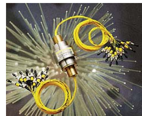
Fig.9 Rotary joints rotating at 100 rpm allowing >10 Gbits per channel transmission at < 2dB loss by using mono-mode fibers, microlens arrays and a Dove prism. [Photo by Schleifring]
