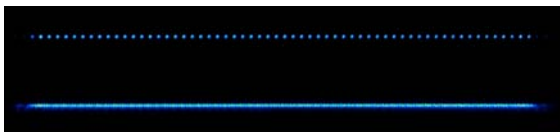
Fig.5 (top) spot pattern from 1D homogenizer and (bottom) using additional linear random diffuser for smoothing.
