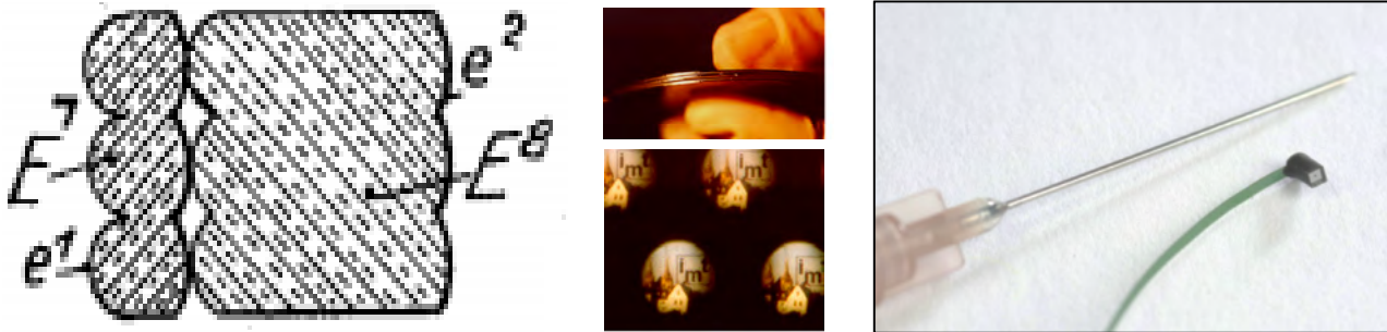
Figure 12. (left) Stack of double-sided microlens arrays as patented by Arnold Arnulf in 1932, (center) a stack of four 100mm microlens wafers serving as 1:1 imaging system for microlens projection lithography, (right) wafer-level camera (NanEye 2B sensor, AWAIBA) serving for disposable endoscopes x .
